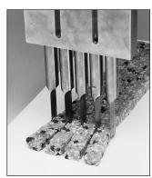
mary principle behind Ultrasonic Food Processing is that a high-frequency vibrating knife (moving at a rate of 20,000 vibrations per second) creates a nearly frictionfree surface between it and the product, resulting in a reduction in sticking problems.
